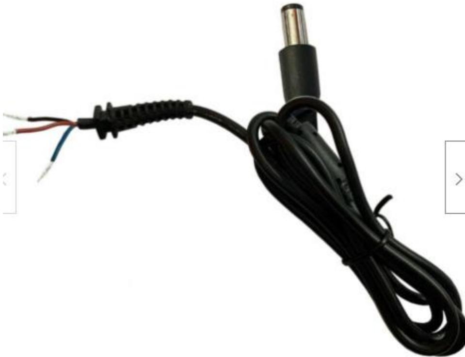
Notice that it has three wires. The red and black are positive and negative as usual. The third wire is something that Dell uses to send a proprietary signal from the power supply to the computer to tell it that a genuine Dell supply is being used, and it's OK to charge the internal battery. Since I couldn't reverse engineer that signal (I hate them!) my adapter only ran the computer but it didn't also charge the internal battery (who cares?)
